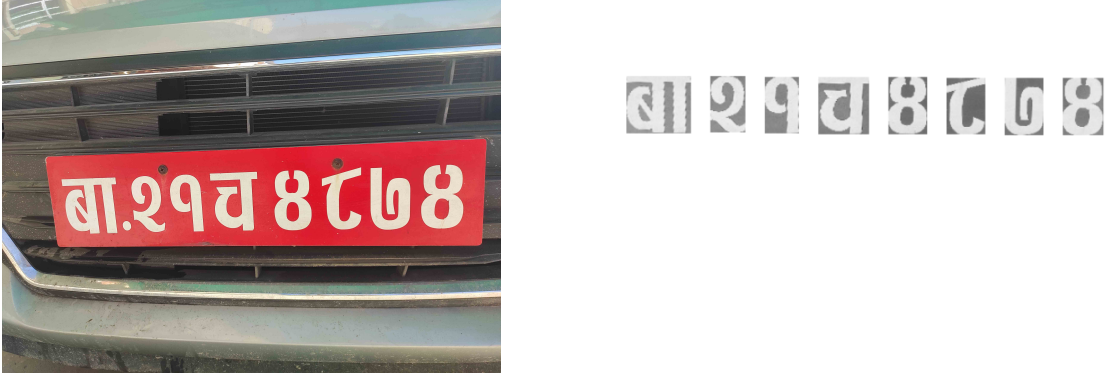
Figure 6.5: Left: Example of image data. Right: Example of segmented character data.
